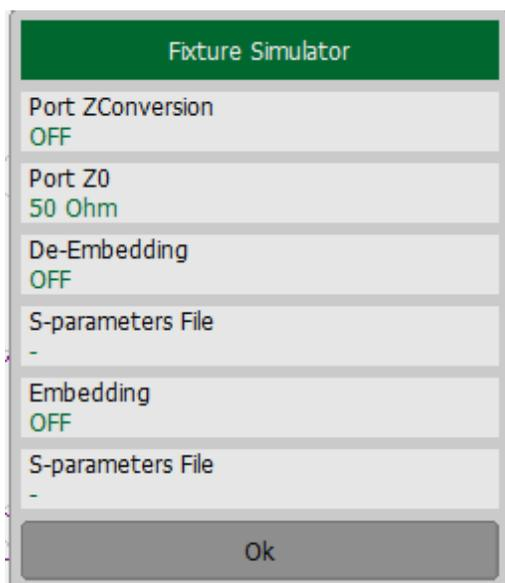
This is the function that converts the S-parameters measured at 50 port into values, which could be determined if measured at a test port with arbitrary impedance.
