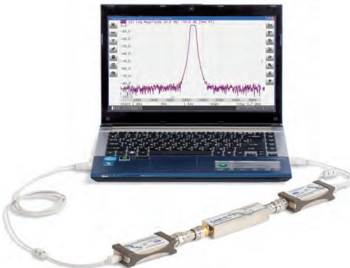
Typical dynamic range of the  $|S_{21}|$  and  $|S_{12}|$  measurements using two 1-Port VNAs is as high as 100 dB, varying by frequency and model. Consult the specifications of each instrument for more detail.
