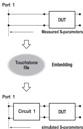
This function allows the user to mathematically simulate the DUT parameters after virtual integration of a fixture circuit between the calibration plane and the DUT. This circuit can be described by an S-parameter matrix in a Touchstone file.
