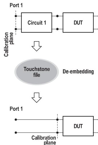
This function allows users to mathematically exclude from the measurement result the effect of the fixture circuit connected between the calibration plane and the DUT. This circuit should be described by an S-parameter matrix in a Touchstone file.
