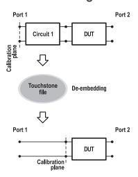
Allows users to mathematically exclude from the measurement result the effect of the fixture circuit connected between the calibration plane and a DUT. This circuit should be described by an S-parameter matrix in a Touchstone file.
