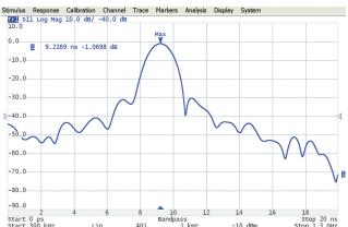
Here, built in time domain analysis allows the user to detect a physical impairment in a cable.
