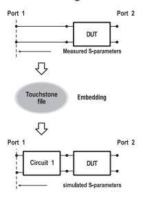
Allows the user to mathematically simulate the DUT parameters after virtual connection through a fixture circuit between the calibration plane and the DUT. This circuit is described by an S-parameter matrix in a Touchstone file.
