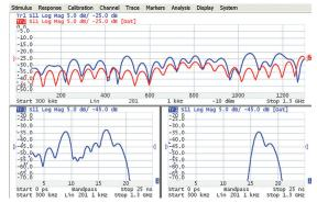
This function applies reverse transformation back to the frequency domain after cutting out the user-defined span in the time domain. Gating filter types are bandpass or notch. For a better tradeoff between gate resolution and level of spurious sidelobes the following filter shapes are available: maximum, wide, normal and minimum.
